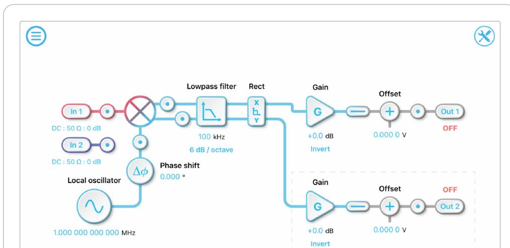
The filtered signal auxiliary output mode generates a second voltage signal proportional to the second low pass filtered output of the demodulator
