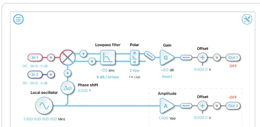
The local oscillator auxiliary output mode will generate a local oscillator at the same frequency as the demodulation waveform with full amplitude and vertical offset control
