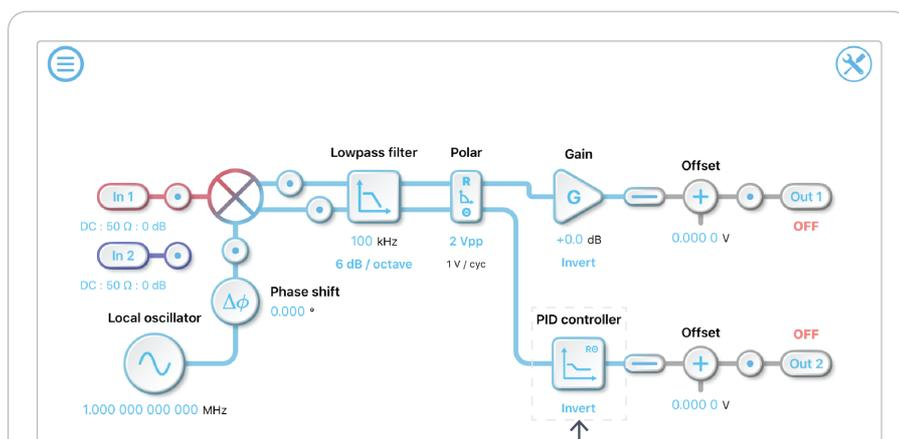
A PID controller can be implemented on the auxiliary output
