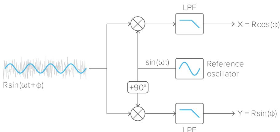
The demodulation process produces two spectral components: an up-shifted signal with a frequency equal to the sum of the input and reference signals, and a down-shifted signal with a frequency equal to the difference of the input and reference signals.
