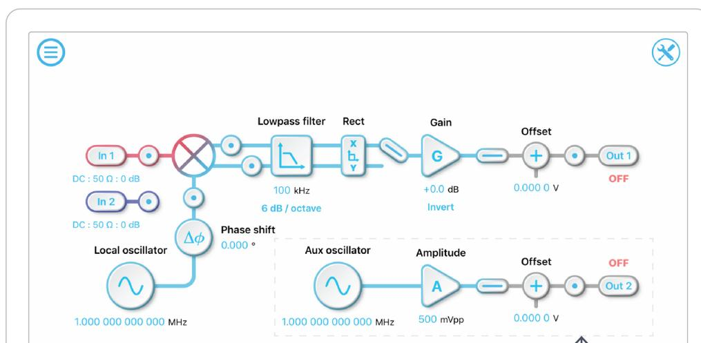
The **aux oscillator** auxiliary output mode allows you to generate a local oscillator signal with independent frequency, amplitude, and vertical offset control
